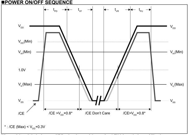
When applying relatively short term VDD pulse whose peak is more than 1.7V, it is required to set falling time, t<sub>VF</sub> more than 0.4ms/V. (In case VDD rises over 1.7V and falls just after that, if this term is short, device may lose its function.)
